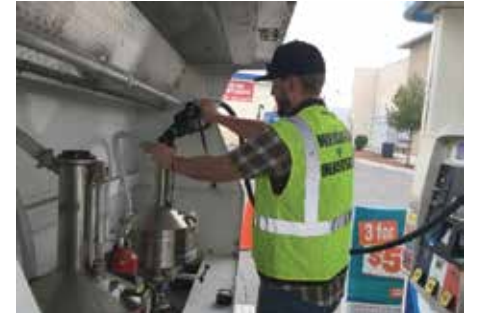
Dispensing into a five-gallon test measure mounted on a prover trailer
